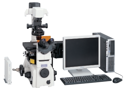
Configuration of DS-5Mc-U2 with biological inverted microscope
